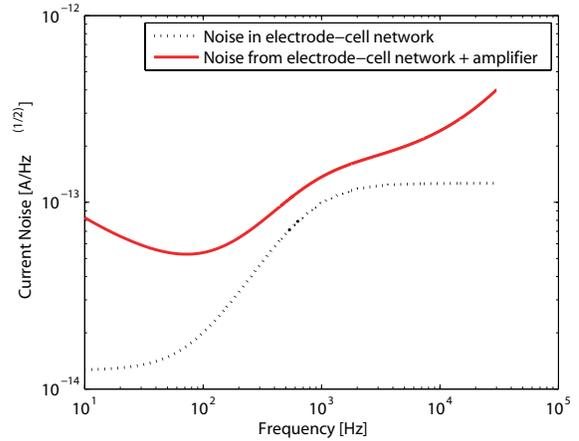
Fig. 11. Current noise spectral density,  $S_P$  of the electrode-cell network compared with the total input referred current noise spectral density,  $SI_{Tot}$ .  $S_P$  is the dominant component of  $SI_{Tot}$  in the recording bandwidth.
