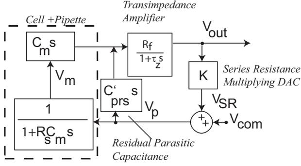
Fig. 7. Block model showing the effect of residual parasitic capacitance on series resistive compensation.
