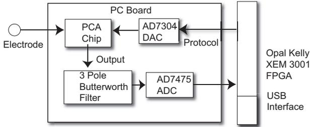
Fig. 13. A block diagram of the hardware test-bed. The test-bed consists of an ADC, a DAC and an anti aliasing filter. The patch-clamp system is controlled using a GUI driven C++ program.
