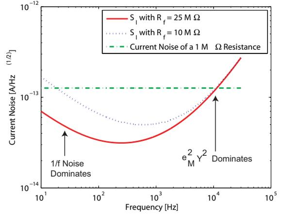
Fig. 10. Electronic noise of the unloaded patch-clamp headstage. The current noise spectral density  $S_I$  is dominated by  $1/f$  noise at low frequencies and at higher frequencies by the voltage noise that is reflected on the input impedance.  $S_I$  has an inverse relationship with the feedback resistance  $R_f$ . When using a  $R_f$  of  $25M\Omega$ , the value of  $S_I$  at  $5kHz$  is comparable to the current spectral density of a  $1M\Omega$  resistance.
