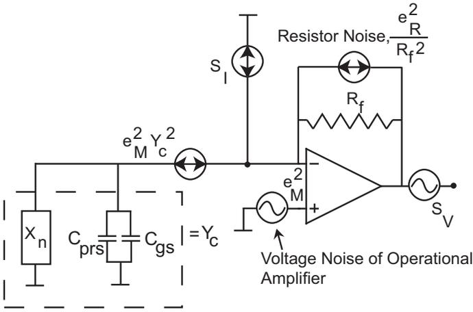
Fig. 9. The model used to calculate the electronic noise of the patch-clamp.
