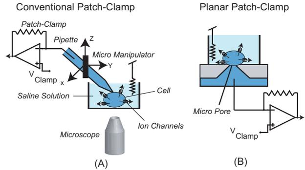
Fig. 1. A. In conventional whole-cell patch-clamp recordings, a pipette filled with electrolyte solution is used as the electrode. It takes considerable skill to attach the pipette to the cell using micro-manipulators and a microscope. B. In planar patch-clamp technology, cells are adhered to an aperture using suction. No micromanipulation is necessary.
