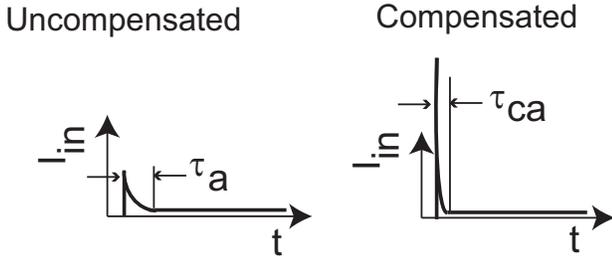
Fig. 5. The series resistance compensation circuit increases the system's bandwidth.
