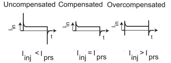
Fig. 6. The capacitive compensation circuit eliminates parasitic overshoots.
