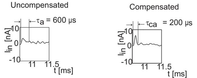
Fig. 17. Measured response of the series resistance compensation circuit. The circuit is able to compensate for up to 70% of  $4M\Omega$  series access resistance.
