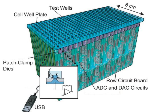
Fig. 2. A high-throughput patch-clamp system comprised of integrated patch-clamp amplifiers and planar electrodes. This system allows to perform simultaneous patch-clamp recordings on an entire 384 well plate.
