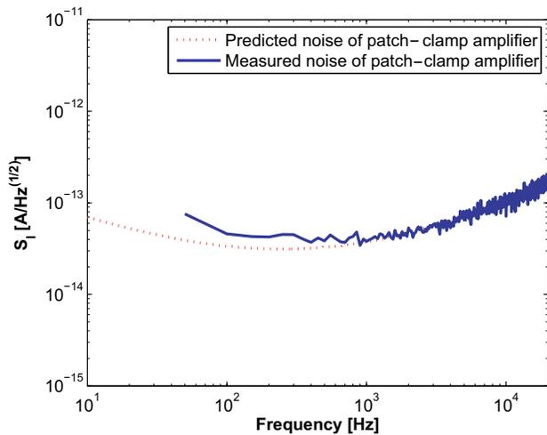
Fig. 19. Measured amplifier input-referred current noise spectral density compared with the theoretical value calculated in equation 16. Integrating the input noise curve yields a rms noise current of 5pA.
