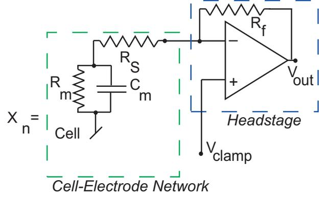
Fig. 8. Electrode plus cell network. The noise level of this network limits the performance of the patch-recording system.
