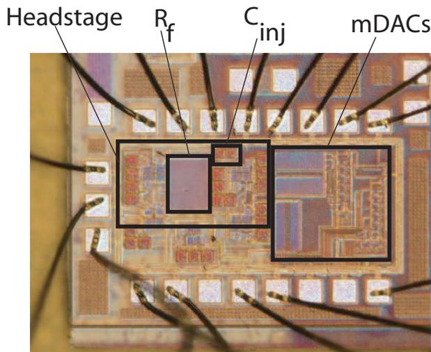
Fig. 20. Die micrograph of the integrated patch-clamp amplifier
