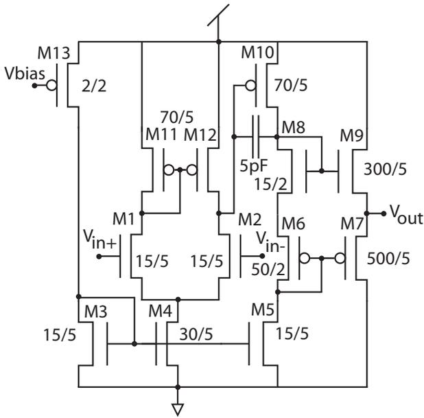
Fig. 12. The operational amplifier used in the design. All ratios [W/L] are given in micron. RN and RP type transistors were used in the design.
