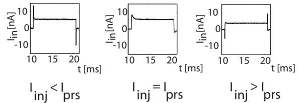
Fig. 18. Measured response of the capacitive compensation circuit. This response was obtained while the circuit compensated a 10pF parasitic capacitance.
