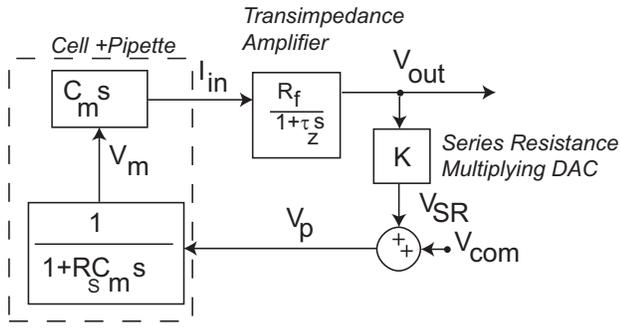
Fig. 4. Block model of the patch-clamp system with series resistance compensation.
