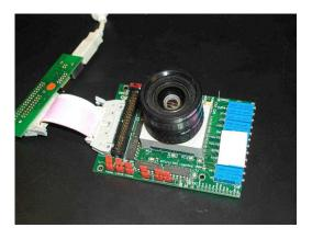
Fig. 2. The  $64 \times 64$  address-event temporal constrast vision sensor used in the fall detector system [17], [18].
