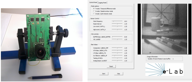
Fig. 10. On the left, experimental setup. On the right, dedicated C++ interface displaying an intensity image taken with indoor illumination of 400\text{lux} .
