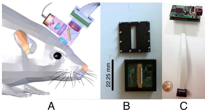
Fig. 1. (A) Head-mountable microscope (B) Our imaging system, placed in a housing to connect to the microscope, measures 22.25 mm x 22.25 mm. (C) Complete imaging system, with a quarter for size comparison. The head-mountable imaging system is connected to the data capture board (about the size of a credit card) via a 20-wire flex cable.
